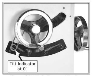
Figure 89. Tilt indicator and scale.
